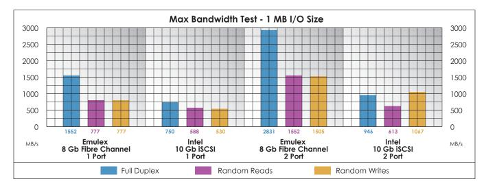
The maximum bandwidth tests show a commanding lead for Fibre Channel. In fact, all three test metrics across either one or two Emulex ports are all very close to the maximum bandwidth potential of this adapter. Intel iSCSI exhibits unexpectedly low single and dual port performance here as well. Across all bandwidth tests, Emulex Fibre Channel is on average of 2 times faster than Intel iSCSI with a maximum 3x bandwidth gain when looking at dual port full duplex performance.
