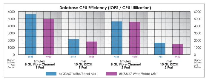
With Windows 2008, Microsoft has included support for MSI-X, which is a recent technology whose goal is to reduce CPU utilization and interrupt time for IOPS intensive environments. Both the Emulex and Intel adapters in our test bed support this feature which addresses the well known issue of IOPS CPU efficiency.
