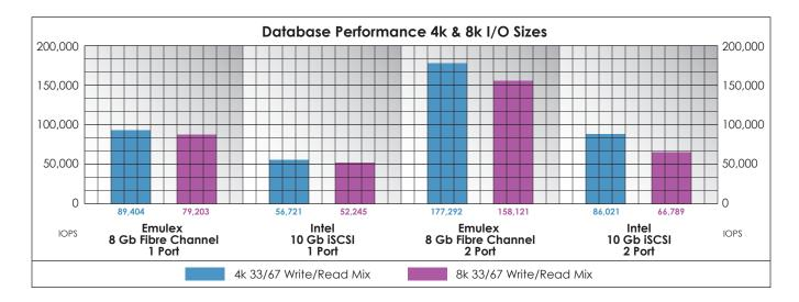
Fibre Channel is the clear winner in 4k and 8k I/O intensive environments. Fibre Channel outperformed iSCSI by an average of 1.9x in our database simulation testing with a maximum performance gain of 2.4x in 8k I/O testing across two ports.
