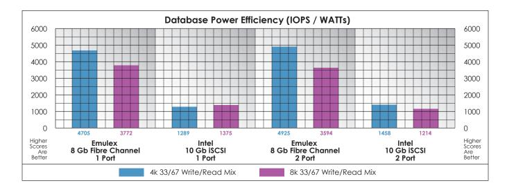
And database power efficiency scales with a significantly better ratio as Fibre Channel is showing a 3.2x average advantage over iSCSI with a maximum 3.7x increase in single port 4k I/O testing.
