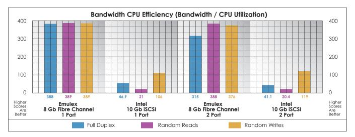
Bandwidth CPU efficiency was determined by simply dividing the bandwidth results by the average CPU utilization of the system taken from Perfmon during each test run. Emulex Fibre Channel showed an average of 10 times the CPU efficiency when performing bandwidth tests against Intel iSCSI with a maximum 19x CPU efficiency gain when looking at dual port random read performance.
